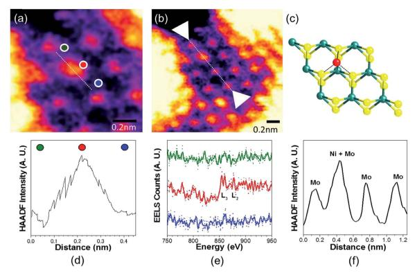
Fig. 4 (a) and (b) HAADF-STEM images of Ni $^{-S}$ MoS<sub>2</sub>. (c) Ni at Mo-atop site model (d) ADF and (e) EELS acquired along the line in b. (f) ADF intensity line profile acquired along the line in b of the Mo sites in  $\langle 100 \rangle$  direction.
