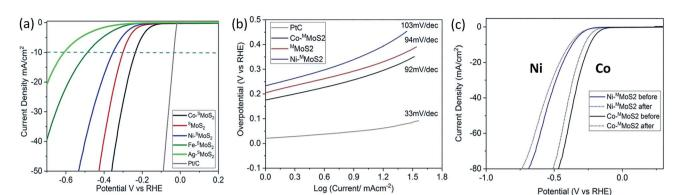
Fig. 2 HER activity analysis by linear sweep voltammography, LSV. (a) LSV of the  $M^{S}MoS_{2}$  nanosheets and the reference 20% Pt/C in 0.5 M  $H_{2}SO_{4}$  at a scan rate of 2 mVs<sup>-1</sup>. (b) Tafel plot of  $Co^{-S}MoS_{2}$ ,  $S^{S}MoS_{2}$ ,  $S^{S}MoS_{2}$ ,  $S^{S}MoS_{2}$  and  $S^{S$
