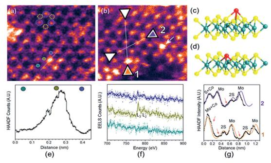
Fig. 3 (a) and (b) HAADF-STEM images of  $Co^{-S}MoS_2$ .<sup>29</sup> Simultaneous acquisition of (c) Co at the Mo-atop site model and (d) Co at the S vacancy site model (e) ADF and (f) EELS acquired along the line in (a). (g) ADF intensity line profiles taken along the numbered lines 1 and 2 shown in (b) ((110) direction). The red arrows in the plot indicate sample drift during image acquisition.
