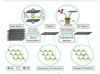
Fig. 1 Synthesis of single-layered MoS<sub>2</sub> (SMoS<sub>2</sub>) and single transitionmetal (TM) atom doped FMoS<sub>2</sub>/SMoS<sub>2</sub>SO<sub>4</sub><sup>2-</sup> groups.
