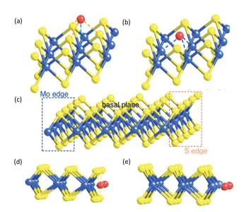
Fig. 5 (a) A metal atom on the Mo top site of  ${}^M\text{MoS}_2$  (b) a metal atom on the S vacancy site of  ${}^M\text{MoS}_2$  (c) the monolayer of perfect triatomic  $\text{MoS}_2$  (d) metal doped S edge of  ${}^M\text{MoS}_2$  (e) metal-doped Mo edge of  ${}^M\text{MoS}_2$ .
