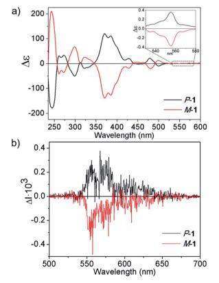
Fig. 5 (a) CD spectra of M-1 and P-1 at  $10^{-5}$  M in  $CH_2Cl_2$ . Inset: CD spectra of M-1 and P-1 in the 530–580 nm region at  $10^{-3}$  M in  $CH_2Cl_2$ . (b) CPL spectra of M-1 and P-1 at  $10^{-5}$  M in CH<sub>2</sub>Cl<sub>2</sub> upon excitation at 372 nm.
