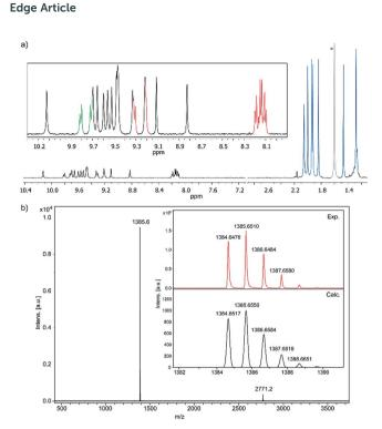
Fig. 2 (a) Partial  $^{1}$ H-NMR spectra (500 MHz,  $C_2D_2Cl_4$ , 293 K) of 1 (see color code in Scheme 1) \*this signal corresponds to residual water. (b) MS and HR-MS (MALDI-TOF) of 1.
