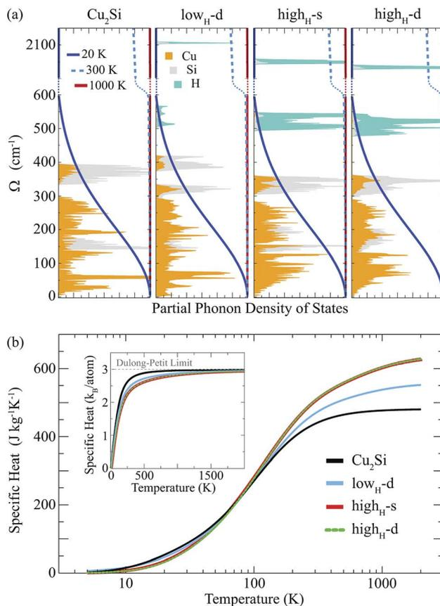
Fig. 4 (a) Phonon partial density of states and derivative of the phonon occupation functions of the  $\text{Cu}_2\text{Si}$  monolayer and its hydrogenated derivatives at various temperatures. Red, light and dark blue lines represent the functions calculated at 1000, 300, and 20 K. (b) For the  $\text{Cu}_2\text{Si}$  monolayer and its hydrogenated derivatives, constant volume specific heat per mass is demonstrated as a function of temperature in logarithmic scale.
