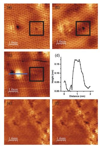
Fig. 6 STM images of graphene from pyridine and benzene grown at 1150 K. (a) As-grown NG, (b) NG after exposure to 10 L of oxygen, (c) NG after exposure to 1010 L of oxygen.  $V_s$ : 100 mV. Black rectangles indicate the defect on the right. (d) Height profile along the blue line in (c). (e) As-grown graphene from benzene. (f) Graphene after exposure to 10 L of oxygen.  $V_s$ : 20 mV.
