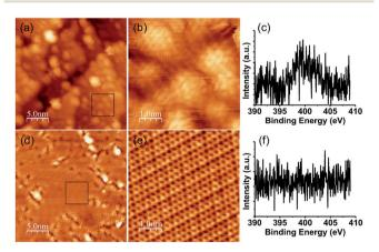
Fig. 1 STM images and XPS spectra of the N 1s region of NG grown (a), (b), (c) at 850 K, (d), (e), (f) at 1000 K. (b) and (e) are magnified images of the black rectangle in (a) and (d), respectively.
