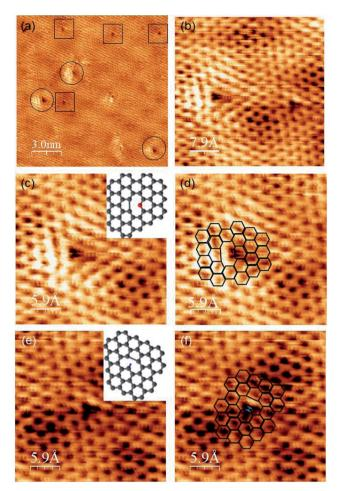
Fig. 5 (a) and (b) STM images of two types of defects in NG grown at 1150 K. V<sub>s</sub>: 10 mV (c) magnified image of left-hand defect in (b), inset: model of the structure. (d) Magnified images with chemical structure. (e) Magnified images of right-hand defect in (b), inset: model of the structure. (f) Magnified image with chemical structure.
