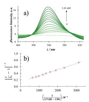
Fig. 2 (a) Fluorescence emission spectra recorded in a  $6\times10^{-5}$  M quercetin aqueous solution containing different CTAB concentrations, within the 0 to 2.45 M range, using an excitation wavelength of 350 nm at  $(28.0\pm0.1)$  °C and the pH  $7\pm0.2$ . (b) Plot [ $I/I_0-1$ ] $^{-1}$  vs. I/[CTAB]-CMC obtained from the fluorescence intensity, I, in (a) and CMC in Table 1.
