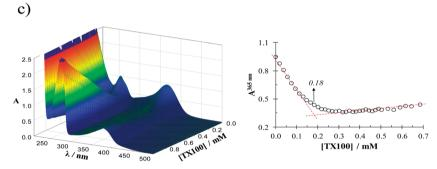
Fig. 1 UV-Vis spectra recorded in the system quercetin– $H_2O$ -surfactant recorded as a function of the concentration of the different surfactants considered: (a) CTAB, (b) SDS and (c) TX-100. In all cases the temperature was  $(28.0 \pm 0.1)$  °C, the pH  $7 \pm 0.2$  and the quercetin concentration was  $5 \times 10^{-5}$  M. The absorbance recorded at 365 nm as a function of the surfactant variation is also shown in each case.
