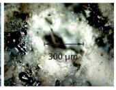
Fig. 5 LIBS measuring spots on an end-of-life refractory brick. Left: refractory brick with three LIBS measuring spots, see white rectangle; bottom, left: broken surface of this material. Middle: enlarged detail corresponding to the white rectangle shown in the left image. Right: detailed view of generated crater with a diameter of about 300 μm. Photos: Fraunhofer ILT.
