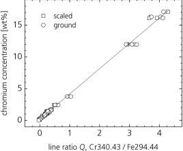
Fig. 8 Analysis curve of chromium for scaled and ground surfaces of steel grades deploying a two phase measuring sequence of laser ablation and LIBS analysis.<sup>2</sup>
