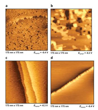
Fig. 4 In situ STM images in BMIPF $_6$  at -0.3 V or -0.4 V for Au(100) (a), Ag(100) (b), Pt(100) (c) and HOPG (d). The images were taken about 30 minutes after assembling the cell.
