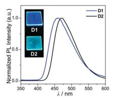
Fig. 4 PL spectra of the film (5 wt% doped on PMMA) for D1 and D2. The insets are photographs of the film under a handheld UV lamp ( $\lambda_{ex}$  = 365 nm).
