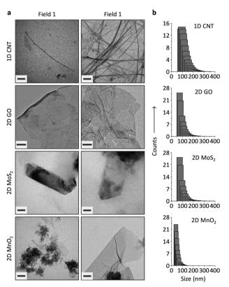
Fig. 2 (a) Transmission electron microscopy (scale bar: 200 nm) and (b) dynamic light scattering of low-dimensional materials including 1D carbon nanotube (CNT,  $0.5 \,\mu g \, mL^{-1}$ ), 2D graphene oxide (GO,  $3 \,\mu g \, mL^{-1}$ ), molybdenum disulphide (MoS<sub>2</sub>, 0.45  $\mu$ g mL<sup>-1</sup>) and manganese dioxide (MnO<sub>2</sub>, 2  $\mu$ g mL<sup>-1</sup>).
