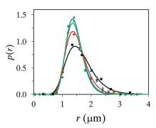
Fig. 6 Size distribution of microcapsules loaded with 0 wt% (■), 10 wt% (●), 25 wt% (♠) and 50 wt% (♦) OIT.
