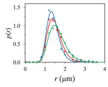
Fig. 7 Size distribution of microcapsules produced with propellant pressures of 2.8  $(\bullet)$ , 2.0  $(\triangle)$ , and 1.4  $(\diamond)$  bar.
