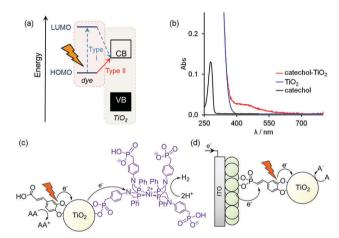
Fig. 1 (a) Energy transfer in Type I (two-step) and Type II (one-step) dyesensitised TiO2 systems; (b) diffuse reflectance absorption spectrum of catechol-modified TiO<sub>2</sub> compared to bare TiO<sub>2</sub> and the transmission spectrum of catechol in water (catechol shown is DHCA); (c) solar H2 production in DSP system (AA = ascorbic acid); (d) layer-by-layer photocathode incorporating catechol $-TiO_2$  (A = acceptor; catechol shown is DHSP).
