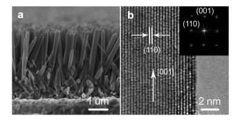
Fig. 1 Morphologies of rutile TiO $_2$  NW arrays. (a) Cross-sectional field emission scanning electron microscopy (FE-SEM) image of NW arrays with an average diameter and length of about 100 nm and 3  $\mu$ m, respectively. (b) High-resolution transmission electron microscopy (HR-TEM) image of a typical NW. The NW has a growth direction of [001] and side surfaces of {110} crystal plane. The inset in panel (b) is the selected area electron diffraction pattern of the NW.
