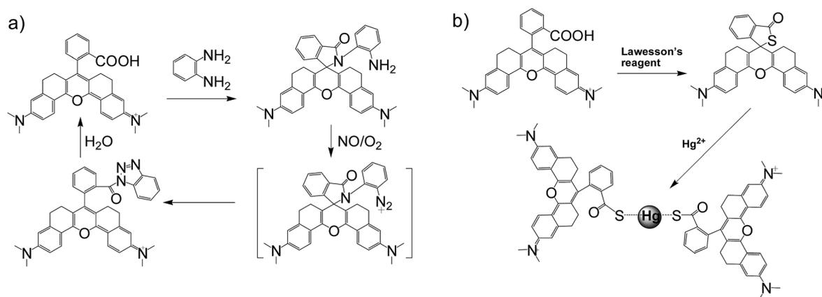
Scheme 2 (a) NO-induced ring opening of **HN7-N2**. (b) Hg<sup>2+</sup>-induced ring opening of **HN7-S**.
