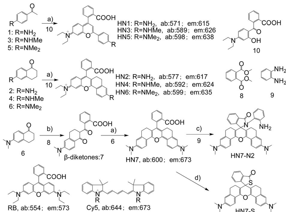
Scheme 1 Synthesis of **HN1–7**, **HN7-N2** and **HN7-S**; structures of classical rhodamine B and Cy5. Conditions: (a) H<sub>2</sub>SO<sub>4</sub>,  $\Delta$ , then 70% HClO<sub>4</sub>; (b) NaH,  $\Delta$ ; (c) DCC/DMAP or POCl<sub>3</sub>/TEA; (d) Lawesson's reagent.
