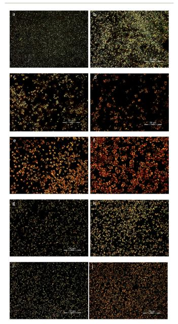
Fig. 9 PLOM photos of (a) PEF at 160 °C, 10 min, (b) PEF at 180 °C, 15 min, (c) PEF at 200 °C, 20 min, (d) PEF at 210 °C, 30 min, (e) PEFSu 92/8 at 150 °C, 20 min, (f) PEFSu 92/8 at 160 °C, 20 min, (g) PEFSu 87/13 at 140 °C, 20 min, (h) PEFSu 87/13 at 160 °C, 20 min, (i) PEFSu 81/19 at 130 °C, 20 min and (j) PEFSu 81/19 at 140 °C, 20 min.
