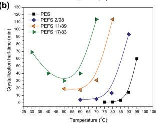
Fig. 5 Isothermal crystallization half-times as a function of temperature: (a) for PEF and EF rich copolymers and (b) for PESu and ES rich copolymers.
