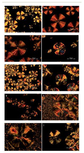
Fig. 10 PLOM photos of (a) PESu at 50 °C, 5 min, (b) PESu at 60 °C, 5 min, (c) PESu at 70 °C, 5 min, (d) PESu at 80 °C, 5 min, (e) PEFSu 2/98 at 50 °C, 5 min, (f) PEFSu 2/98 at 60 °C, 7 min (g) PEFSu 11/89 at 60 °C, 7 min, (h) PEFSu 11/89 cooled to room temperature after crystallization at 60 °C for 7 min, (i) PEFSu 11/89 cooled to room temperature after crystallization at 60 °C for 7 min and (j) PEFSu 17/83 at 50 °C, 10 min.
