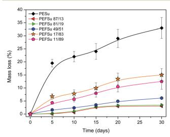
Fig. 11 Weight loss plots during enzymatic hydrolysis.
