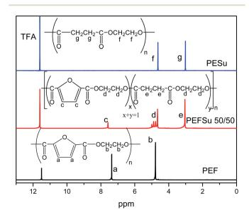
Fig. 1 Chemical structures and <sup>1</sup>H NMR spectra of PEF, PESu and the PEFSu 50/50 copolymer.
