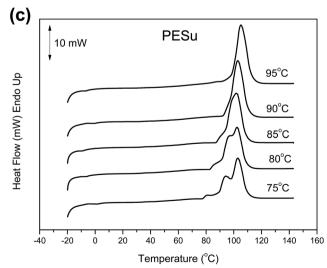
**Fig. 6** DSC traces of (a) PEFSu 92/8, (b) PEFSu 17/83 and (c) neat PESu samples crystallized at different temperatures.
