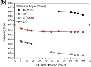
Fig. 7 (a) WAXD patterns of the PEFSu copolymers and the PEF and PESu homopolymers, (b) variation of the interplanar distances (*d*-spacing) with the composition of PEFSu copolymers.
