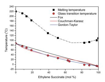
Fig. 4 Variation of the melting temperature  $(T_{\rm m})$  and glass transition temperature  $(T_{\rm g})$  of the PEFSu copolymers with composition.
