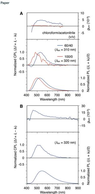
Fig. 5 PL (bottom), CPL (middle) and  $g_{lum}$  (top) spectra of poly-9 (1.0  $\times$  10<sup>-4</sup> M) in chloroform/acetonitrile (100/0 or 60/40, v/v) (A) and of a chloroform-cast film of poly-9 after exposure to acetonitrile vapor for 96 h (B) at room temperature. The corresponding PL (not normalized) and CPL (unprocessed) spectra are shown in Fig. S14.†
