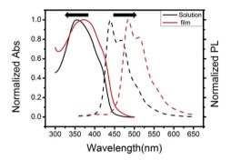
Fig. 2 Normalized UV-vis absorption and fluorescence spectra of 3,6-Cbz-EDOT in CH<sub>2</sub>Cl<sub>2</sub> measured at 10<sup>-6</sup> M repeat unit<sup>-1</sup> and in thin films.
