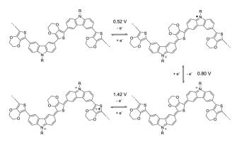
Schematic illustration of the stepwise oxidation of 3,6-Cbz-EDOT.
