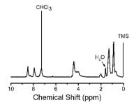
Fig. 1 <sup>1</sup>H NMR of 3,6-Cbz-EDOT in CDCl<sub>3</sub>.
