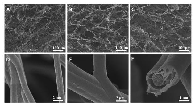
Fig. 2 SEM images of original sponge 1 (A,  $8.42 \text{ mg cm}^{-3}$ ), sponge 2 (B,  $7.43 \text{ mg cm}^{-3}$ ), sponge 4 (C,  $5.16 \text{ mg cm}^{-3}$ ), higher magnification of sponge 4 (D), sponge 4 coated with 1000 nm PPX (E, sponge 4–1000), and the corresponding cross section of sponge 4–1000.
