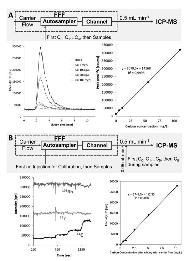
Fig. 6 Experimental setup, calibration raw data and calibration curves both for the flow injection calibration (A) and for the post-channel calibration (B) approach using the example of the soil extracts
