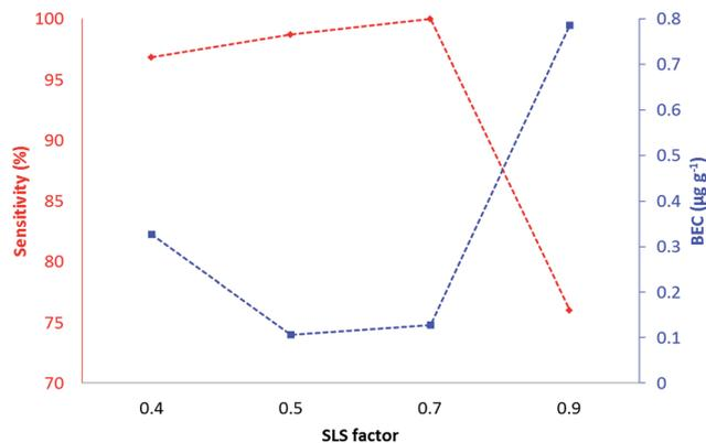
Fig. 1 Influence of the SLS-factor on the background and the sensitivity of  $m/z$  63,  $SLG = 0.9$ . The same trend was observed for all masses. The lowest background and the highest sensitivity was at a SLS-factor of 0.7. All data was normalised to the calibration curve with the greatest slope.
