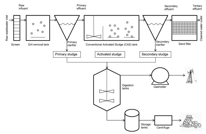
Fig. 1 Typical waste water treatment plant processes.
