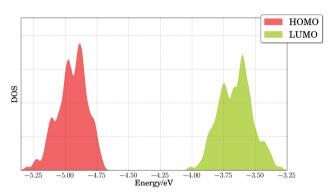
Fig. 6 Density of states (DOS) of calculated PBE HOMO and LUMO energy levels for PTB7 extended chains. A Gaussian broadening of 0.02 eV was used in smoothing the results.
