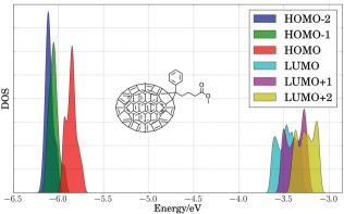
Fig. 5 Density of states (DOS) of calculated B3LYP HOMO-2, HOMO-1, HOMO, LUMO, LUMO+1, and LUMO+2 energy levels (eV) for 80 PC71BM configurations, with each energy level marked by color. A Gaussian broadening of 0.02 eV was applied to computed energy levels
