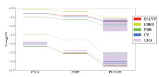
Fig. 3 Calculated (PBE, PBE0, and B3LYP levels of theory) and experimental (cyclic voltammetry/CV and ultraviolet photoelectron spectroscopy/UPS) HOMO and LUMO energy levels for ternary system of PTB7, PID2, and PC71BM.
