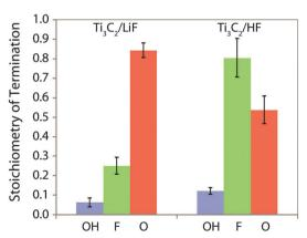
Fig. 3 Composition of the  $Ti_3C_2T_x$  surface functional groups produced by etching of the Ti<sub>3</sub>AlC<sub>2</sub> in HF and LiF-HCl solutions, per Ti<sub>3</sub>C<sub>2</sub> formula unit, i.e.  $Ti_3C_2(OH)_xF_yO_z$
