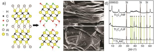
Fig. 1 (a) Schematic of etching from  $Ti_3AlC_2$  to  $Ti_3C_2T_x$  showing terminations and interlayer water. Typical SEM micrographs of (b) HF-etched  $Ti_3C_2T_x$ showing accordion-like structure and (c) LiF-HCl etched  $Ti_3C_2T_x$ , with a more compact structure. (d) XRD patterns of  $Ti_3AlC_2$  and  $Ti_3C_2T_x$  etched with HF or LiF-HCI. Green vertical lines denote the presence of MAX phase peaks, and grey regions are peaks from crystalline Si 10 wt% internal standard
