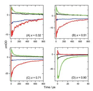
Fig. 5 Kinetic traces extracted from transient PSCP broadband absorption spectra for (MAI)<sub>x</sub>(PbI<sub>2</sub>)<sub>1-x</sub>/TiO<sub>2</sub>/glass samples. Panels (A–D) are for  $x=0.32,\,0.51,\,0.71$  and 0.90, respectively. Black and green lines are for 2 and 50 μJ cm $^{-2}$  fluence at  $\lambda_{probe}=600$  nm. Blue and red lines represent 2 and 50 μJ cm $^{-2}$  fluence at  $\lambda_{probe}=750$  nm.
