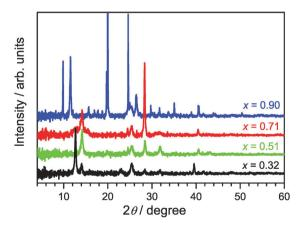
Fig. 1 XRD patterns of  $(MAI)_x(PbI_2)_{1-x}/TiO_2/glass$  samples as a function of the initial mole fraction x of MAI. The materials were deposited by a single-step deposition process from DMF. Black, green, red and blue lines are the XRD patterns for x=0.32, 0.51, 0.71 and 0.90, respectively.
