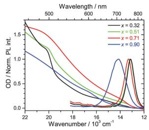
Fig. 2 Steady-state absorption (left) and photoluminescence spectra (right) of  $(MAI)_x(PbI_2)_{1-x}/TiO_2/glass$  prepared using different initial mole fractions x of MAI. Black: 0.32, green: 0.51, red: 0.71, blue: 0.90. For the sake of an easier comparison, absorption spectra are set to zero at 840 nm. Photoluminescence spectra are normalized to their peak amplitude.
