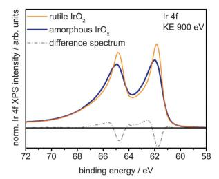
Fig. 1 Ir 4f spectra and difference spectrum of rutile IrO<sub>2</sub> and amorphous IrO<sub>x</sub> measured in UHV at a kinetic energy of the photoelectrons of 900 eV.
