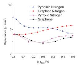
Fig. 9  $\,$  Total differential capacitance of different types of N-doped graphene for the 1 M NaCl aqueous electrolyte.
