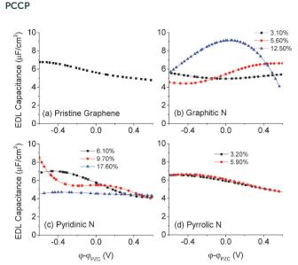
Fig. 8 Electric double-layer (EDL) capacitance of (a) pristine graphene, (b) graphitic, (c) pyridinic and (d) pyrrolic nitrogen-doped single layer graphene with different doping concentrations. The EDL capacitance is obtained from classical MD simulation for the 1 M NaCl aqueous electrolyte.
