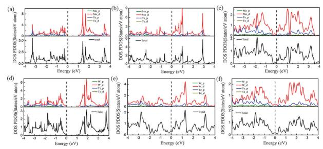
Fig. 6 Density of states (DOS) and partial density of states (PDOS) of monolayer MoTe<sub>2</sub> with 2H (a), 1T (b) and 1T' (c) phases and that of monolayer WTe<sub>2</sub> with 2H (d), 1T (e) and 1T' (f) phases. Note that the perpendicular dashed line at 0 eV denotes the Fermi level
