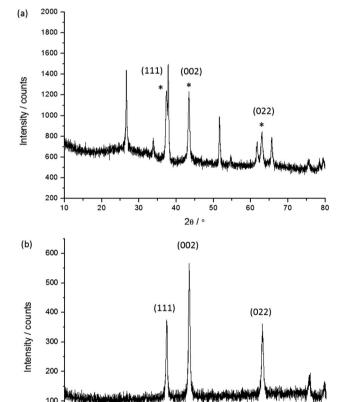
**Fig. 5** Representative X-ray diffraction patterns for sample **4**: (a) the NiO film on FTO; (b) the NiO nanoparticles removed from the film. The diffraction peaks indexed with the (*hkl*) notation correspond to the main NiO phase.<sup>25</sup> \* Denotes the peaks corresponding to NiO.
