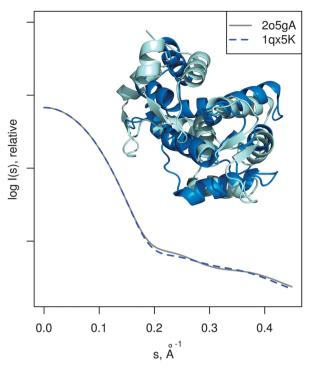
**Fig. 5** Limitations of the approach. Two known structures of calmodulin in different conformation are shown superimposed, even though they differ considerably (RMSD is 10.2 Å). The corresponding theoretical SAXS profiles are very similar, meaning that in this case SREFLEX will not be able to model the conformational change as explained in the text.
