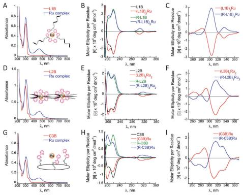
Fig. 2 UV-Vis and CD spectra measured at rt. in acetonitrile: (A, D and G) UV-Vis spectra of L1B (50 μM), L2B (50 μM), C3B (17 μM) and their Ru<sup>2+</sup> complexes (17 µM each) respectively. (B, E and H) CD spectra of L1B, L2B, C3B (100 µM each) and their Ru2+ complexes (30 or 100 µM each), respectively. (C, F and I) CD spectra of (L1B)<sub>3</sub>Ru and (L2B)<sub>3</sub>Ru<sub>2</sub>, and (C3B)Ru (200 μM each), respectively
