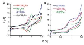
Fig. 3 Comparison between the cyclic voltammograms of (A) 0.5 mM intermolecular Ru complexes and (B) 0.5 mM (L1B)<sub>3</sub>Ru and (C3B)Ru and 0.25 mM (L2B)<sub>3</sub>Ru<sub>2</sub> that were recorded in acetonitrile at rt. using a glassy carbon working electrode, platinum counter electrode, and Ag/AgNO<sub>3</sub> reference electrode. Scan rate: 100 mV s<sup>-1</sup>.
