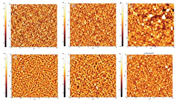
Fig. 6 Tapping-mode 2.5 × 2.5 μm AFM topographies of films of QNC (top panels) and EPI (bottom panels): (a, d) pristine evaporated films; (b, e) SUB functionalized films; (c, f) bacterial RC on SUB functionalized films after washing with buffer solution.
