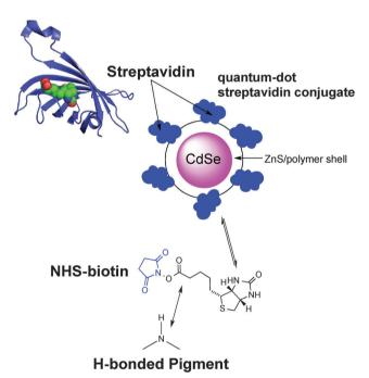
Fig. 3 The structure of the monomeric streptavidin protein with a bound biotin molecule; along with the qdot-705 luminescence label structure. The NHS-biotin linker is used to biotinylate the hydrogen-bonded semiconductor surface, affording specific binding sites for streptavidin.
