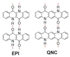
Fig. 1 Molecular structures of hydrogen-bonded pigments epindolidione (EPI) and guinacridone (QNC). Red dashed lines indicate intermolecular hydrogen-bonding.
