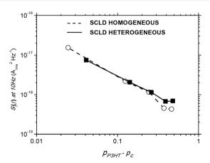
Fig. 5 Noise power spectral density at 10 Hz as a function of  $(p_{P3HT} - p_C)$ for heterogeneous (solid) and homogeneous (open) SCLDs.
