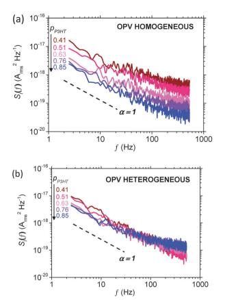
Fig. 7 1/f noise spectra for (a) homogeneous and (b) heterogeneous P3HT:PCBM OPVs with various blend ratios:  $p_{P3HT} = 0.41$  (brown), 0.51 (red), 0.63 (pink), 0.76 (purple) and 0.85 (blue)
