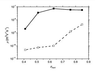
Fig. 3 Hole mobility in the P3HT:PCBM blends as a function of P3HT volume percentage (pP3HT) for heterogeneous (solid line) and homogenous (dashed line) morphologies.
