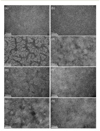
Fig. 1 TEM images of the P3HT:PCBM blends: (a) and (b)  $p_{P3HT} = 0.41$ , (c) and (d)  $p_{P3HT}$  = 0.51, (e) and (f)  $p_{P3HT}$  = 0.63, (g) and (h)  $p_{P3HT}$  = 0.85; with thermal treatments: left column (a)-(g) corresponds to heterogeneous active layers, while right column (b)-(h) corresponds to homogeneous
