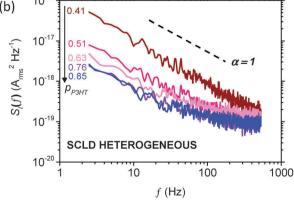
Fig. 4 1/f noise spectra for (a) homogeneous and (b) heterogeneous P3HT:PCBM SCLDs with  $p_{P3HT} = 0.41$  (brown), 0.51 (red), 0.63 (pink), 0.76 (purple) and 0.85 (blue).
