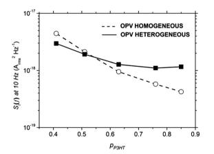
Noise spectral density measured at 10 Hz as a function of  $p_{P3HT}$ .
