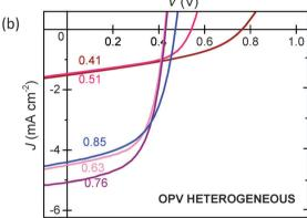
Fig. 6 J-V characteristics of (a) homogeneous and (b) heterogeneous P3HT:PCBM OPVs under AM1.5 illumination with various blend ratios:  $p_{P3HT} = 0.41$  (brown), 0.51 (red), 0.63 (pink), 0.76 (purple) and 0.85 (blue).
