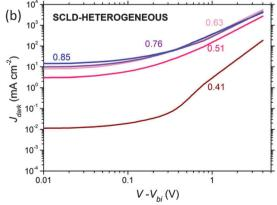
Fig. 2 J-V characteristics under dark conditions for hole-only SCL P3HT:PCBM diodes for (a) homogeneous and (b) heterogeneous active layers, and blend ratios:  $p_{P3HT} = 0.41$  (brown), 0.51 (red), 0.63 (pink), 0.76 (purple) and 0.85 (blue)
