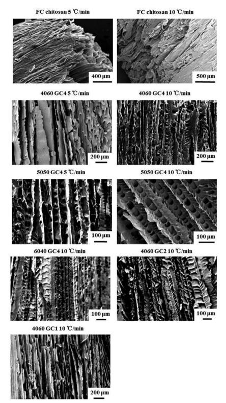
Fig. 7 SEM images of freeze cast scaffolds fabricated with various compositions and cooling rates. Cross-sections parallel to the freezing direction, which show the oriented pore structures.
