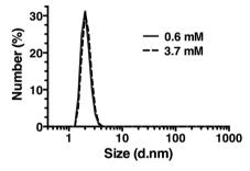
Fig. 7 Dynamic light scattering of R5 solutions. R5 is monodisperse at all concentrations tested with a single peak centered at a hydrodynamic diameter of 2 nm. Representative results at the lowest and highest concentrations tested are shown.
