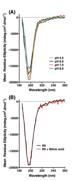
Circular dichroism spectra of R5. (A) Peptide ellipticity is characteristic of random coil at all pH values tested. (B) Peptide ellipticity is unchanged in the presence of silicic acid at pH 7.0.
