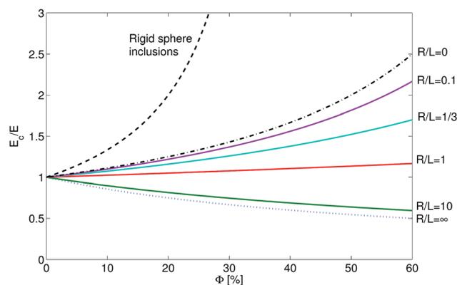
Fig. 4 The stiffness of soft composites. Young's modulus of composites of droplets embedded in linear-elastic solids,  $E_c$  as a function of liquid content. The dotted curve shows Eshelby's prediction without surface tension. The dash-dotted curve shows the surface-tension dominated limit,  $R/L \ll 1$ . The dashed curve shows Eshelby's prediction for rigid spheres embedded in an elastic solid.
