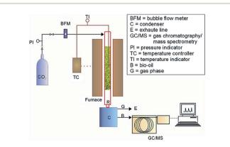
**Fig. 5** Schematic reactor system for microalgae pyrolysis.<sup>56</sup> Copyright 2012 Elsevier.
