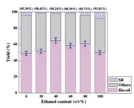
**Fig. 12** Effect of ethanol content on the bio-oil, others and SR yields for the microalgae liquefaction in ethanol-water cosolvent.<sup>175</sup> Copyright 2012 Elsevier.
