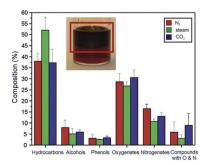
Fig. 7 Bio-oil composition of pyrolysis employed at three atmospheres: N<sub>2</sub>, steam, and CO<sub>2</sub> (ref. 111). Copyright 2012 Elsevier. Process conditions: 773 K, N<sub>2</sub> flow = 250 mL min<sup>-1</sup>, algae mass = 7 g, dp < 90 mm.
