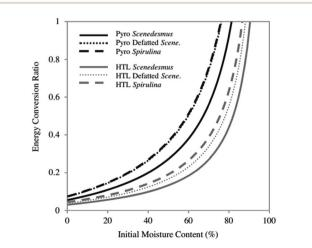
Fig. 18 ECR for HTL and pyrolysis of algal biomass at varying initial moisture contents.<sup>86</sup> Copyright 2012 Elsevier.
