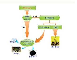
Fig. 4 Possible microalgal processing options based on lipid content.
