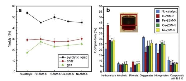
Fig. 8 Experimental results of catalytic pyrolysis reactions conducted using different zeolites.<sup>111</sup> Copyright 2012 Elsevier. (a) Effect of catalyst on product yield in catalytic pyrolysis reactions. (b) Bio-oils product distribution. Process conditions: 773 K, N<sub>2</sub> flow = 250 mL min<sup>-1</sup>, algae mass = 7 g, WHSV = 13.5 h<sup>-1</sup>, GHSV = 20 000 h<sup>-1</sup>, residence time ~1.5 s.
