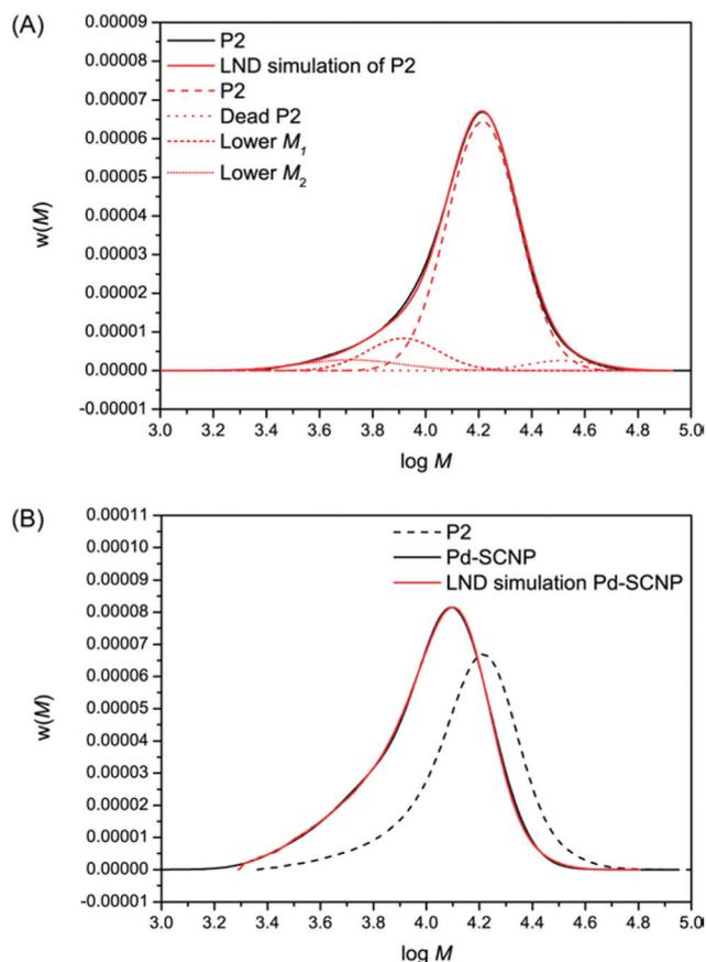
**Fig. 4** Experimental SEC (DMAC, RI) data and corresponding log-normal distribution (LND) simulations. (A) Black trace: experimental **P2**, red trace: LND fit of **P2** using 4 distributions, namely **P2** (red dashed), dead **P2** (red dotted), lower  $M_1$  (red short dashed), and lower  $M_2$  (red long dashed). (B) Black trace: experimental **Pd-SCNP**, red trace: LND fit of **Pd-SCNP** using 7 distributions, black dashed trace: experimental **P2** for comparison.
