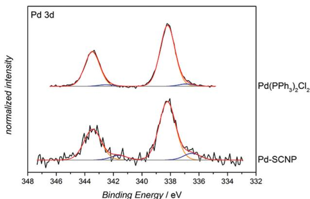
**Fig. 5** Pd 3d XPS spectra of **Pd-SCNP** (bottom) and  $[\text{Pd}(\text{PPh}_3)_2\text{Cl}_2]$  (top). The comparison of the prepared SCNPs with the model complex shows that the binding energy of the main Pd species at 338.2 eV in **Pd-SCNP** is in excellent agreement with the binding energy in  $[\text{Pd}(\text{PPh}_3)_2\text{Cl}_2]$ .
