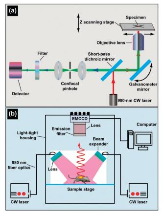
Fig. 22 Schematic setup used for in vitro and in vivo imaging of cells and animals. (a) Schematic illustration of a laser scanning UC luminescence confocal microscope for in vitro study. (b) Experimental setup for in vivo imaging of small animals using UC nanocrystals as biomarkers. (Reprinted with permission from ref. 173 and 246. Copyright 2009, American Chemical Society.)
