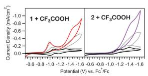
Fig. 3 Acid titrations of 0.5, 4, and 10 eq. of [CF<sub>3</sub>COOH] into equimolar solutions of 1 and 2 (0.39 mM). The black traces are the respective acidfree voltammograms. Voltammograms recorded at 100 mV s<sup>-1</sup> in 100 mM [Bu<sub>4</sub>N][PF<sub>6</sub>] CH<sub>3</sub>CN solutions.
