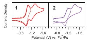
Fig. 2 Cyclic voltammograms of 0.20 mM  $\bf 1$  and  $\bf 2$  without acid at 100 mV s<sup>-1</sup> and with 0.1 M  $[Bu_4N][PF_6]$ . The  $Ni^{II}/Ni^{II}$  reduction of  $\bf 1$  is reversible (dotted trace) and the Ni<sup>1</sup>/Ni<sup>0</sup> reduction is guasi reversible. The Ni<sup>11</sup>/Ni<sup>1</sup> reduction of 2 is reversible (dotted trace); however the Ni<sup>1</sup>/Ni<sup>0</sup> reduction is irreversible.
