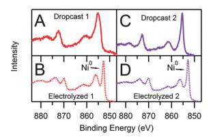
Fig. 4 High resolution XPS spectra of the Ni 2p region. (A) Dropcast 1 onto gold plated silica wafer. (B) Electrolyzed 1 on a glassy carbon plate from a 0.38 mM  $\bf 1$  and 13.6 eq. CF<sub>3</sub>COOH solution. (C) Dropcast  $\bf 2$  onto gold plated silica wafer. (D) Electrolyzed 2 on a glassy carbon plate from a 0.38 mM 2 and 13.6 eq. CF<sub>3</sub>COOH solution. Electrolyzed solutions contained 0.1 M [Bu<sub>4</sub>N][PF<sub>6</sub>] and were held at -1.66 V vs. Fc<sup>+</sup>/Fc for 480 s.
