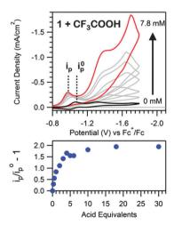
Fig. 1 Top: voltammograms of 0.39 mM 1 with additions of 0 to 20 eq.  $(7.8 \text{ mM}) \text{ of } \text{CF}_3\text{COOH at } 100 \text{ mV s}^{-1} \text{ in a } 100 \text{ mM } [\text{Bu}_4\text{N}][\text{PF}_6] \text{ CH}_3\text{CN}$ solution. Bottom: the peak current of the prewave relative to the oneelectron reduction of the catalyst in the absence of acid ( $i_p$  = peak current,  $i_p^0$  = peak current of Ni<sup>II</sup>/Ni<sup>I</sup> reduction in absence of acid).
