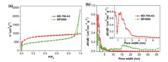
Fig. 2 (a)  $N_2$  physisorption isotherms (77 K) and (b) NL-DFT pore size distributions (PSD) of BD-700-A3 and BP2000, inset is the PSD of BD-700-A3 in the range from 0.5 to7 nm.
