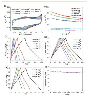
Fig. 4 Electrochemical performance of BD-700-A3 based on the three-electrode system: (a) CVs at various scan rates; (b)  $C_s$  at various current densities, compared with commercially available carbon BP2000 and some other bean dregs derived carbons; (c–e) galvanostatic charge/discharge curves collected at various current densities ( $I_s$ ); (f) capacitance retention measured at 5 A  $g^{-1}$ .
