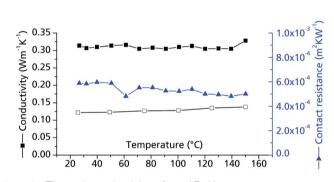
Fig. 10 Thermal conductivity of  $\mu$ p-AF. Measurements were conducted on bulk  $\mu$ p-AF (pellet,  $\emptyset = 12.68$  mm, h = 1.71 mm, forming pressure = 13 kN;  $\rho = 0.714$  g cm<sup>-3</sup>, empty symbols) and a  $\mu$ p-AF@Al coated sheet with protective layer (filled symbols). For the  $c_{\rm p}$  values, the curve determined for bulk  $\mu$ p-AF was used in both cases (see Fig. S3 in ESI†).
