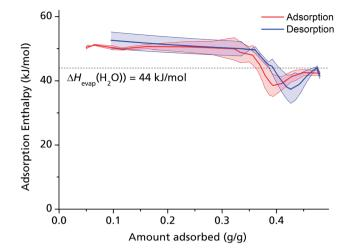
**Fig. 4** Heat of adsorption for  $\mu$ p-AF–water, calculated from 298 K, 313 K and 333 K isotherms. The shaded area indicates the standard deviation of the respective linear fits through the points  $P_1$ ,  $P_2$ ,  $P_3$ .
