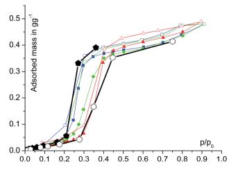
**Fig. 3** Water sorption *isotherms* of bulk µp-AF, acquired at 25 °C water  $p_0 = 3.17$  kPa, (**m**), 40 °C ( $p_0 = 7.39$  kPa, (**o**) and 60 °C  $p_0 = 19.95$  kPa, (**a**), and *isobars* at 1.2 kPa (**b**) and 5.6 kPa (O). Adsorption is depicted with filled, desorption with empty symbols.
