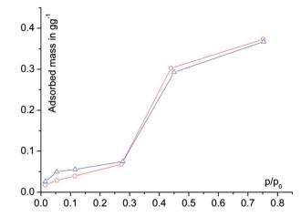
Fig. 9 Equilibrium water desorption isobars of a representative  $\mu$ p-AF@Al coating after 1500 ( $\odot$ ) and 4500 cycles ( $\triangle$ ). Isobars were acquired gravimetrically under pure water vapour atmosphere, at  $p_{H_2O} = 5.6$  kPa, with 140 °C  $\geq T \geq 40$  °C. Samples were degassed at 150 °C under vacuum for 12 h prior to measurement, and loaded with water vapour for 8 h. Adsorbed mass is based on the amount of  $\mu$ p-AF coating.
