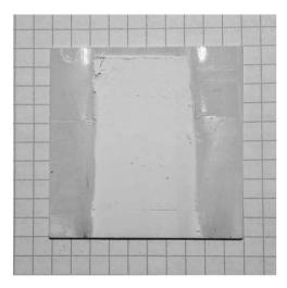
Fig. 6 Representative image of an  $\mu$ p-AF@Al coated aluminium sheet. Edges were covered by mounting clamps during coating synthesis.
