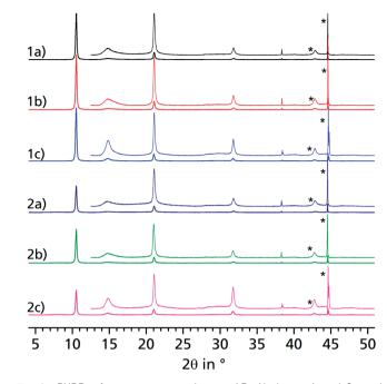
Fig. 8 PXRD of two representative  $\mu$ p-AF@Al sheets 1 and 2, each before cycling (a), after 1500 (b) and 4500 (c) ad-/desorption cycles with water vapour. Sheet 2 has been covered with the silicon resin. Insets are multiplied by the factor of 6 for better visualization. Peaks marked with an asterisk ( $\star$ ) are caused by the Al substrate.
