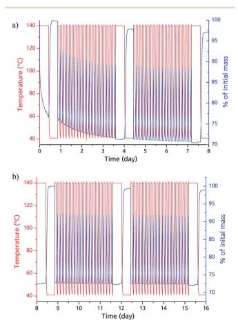
Fig. 5 Thermogravimetric adsorption/desorption cycling experiments for 40 cycles (a), and another 40 cycles (b) of bulk  $\mu$ p-AF. Long segments at the beginning, in the middle and at the end of each experiment were conducted to determine the equilibrium loading of the sample.
