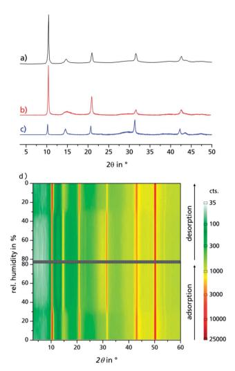
Fig. 2 PXRD of bulk  $\mu$ p-AF as extracted from patent literature (a), dried  $\mu$ p-AF (stored at 120 °C under vacuum for 24 h (b)) and hydrated  $\mu$ p-AF (stored under 100% water vapour atmosphere overnight, (c)). (d) Reversible structural transition observed by *in situ* PXRD in a humidity chamber at 313 K. See Fig. S5 in the ESI† for the individual diffractograms.
