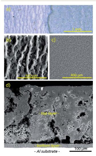
Fig. 7 (a) Representative optical microscope image of the  $\mu$ p-AF@Al coating in top-down view, with the top layer being removed in the right part of the image in order to expose the bottom layer. The different structures can be seen in (b) (SEM image of the top-down view of the top layer) and (c) (SEM image of the top-down view of the bottom layer), and in the polished cross-section of the whole coating (d).
