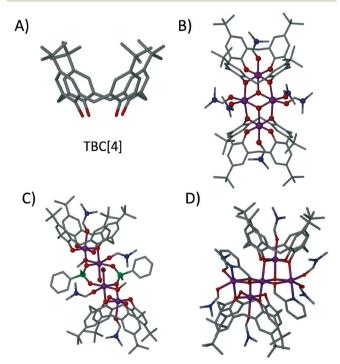
Fig. 1 A)  $p^{-t}$ Bu-calix[4]arene, TBC[4]. B) TBC[4]-supported  $[Mn^{||}_{2}Mn^{||}_{2}]$ SMM motif. 4b,c C) Phenylphosphinate-bridged dimer of TBC[4]-supported [Mn $^{\rm III}$ Mn $^{\rm III}$ ] dimers. $^{\rm 4e}$  D) TBC[4]-supported Mn $^{\rm III}_3$ Mn $^{\rm II}_2$  cluster formed with hmp as an ancillary ligand. 4 Colour code: C - grey, O - red, N - royal blue, Mn - purple, P - green. H atoms are omitted for clarity. Figures not to scale.
