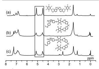
**Fig. 1** <sup>1</sup>H NMR spectra of (a) DecaF-Benz, (b) OctaF-PolyBenzPre and (c) Tetra-decaF-PolyBenzPre in CDCl<sub>3</sub>.
