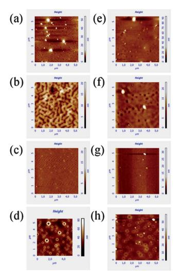
Fig. 8 AFM height pictures of the precursor films before (a-d) and after curing (e-h). Before curing: (a) nonF-PolyBenzPre, (b) HexaF-PolyBenzPre, (c) OctaF-PolyBenzPre, (d) TetradecaF-PolyBenzPre. After curing: (e) nonF-PolyBenzPre, (f) HexaF-PolyBenzPre, (g) OctaF-PolyBenzPre, (h) TetradecaF-PolyBenzPre.
