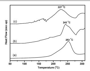
**Fig. 4** DSC thermograms of (a) BisF-Benz, (b) nonF-PolyBenzPre and (c) HexaF-PolyBenzPre.
