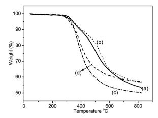
Fig. 5 TGA thermograms of cured (at 250 °C for 0.5 h) prepolymers (a) OctaF-PolyBenzPre, (b) TetradecaF-PolyBenzPre, (c) nonF-PolyBenzPre and (d) HexaF-PolyBenzPre
