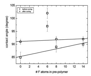
**Fig. 7** The change of water contact angles on thin films of polymeric benzox-azine precursors as a function of the number of F atoms in the precursor. Before curing  $(\Box)$ , after curing  $(\bigcirc)$ , and error bars (I).
