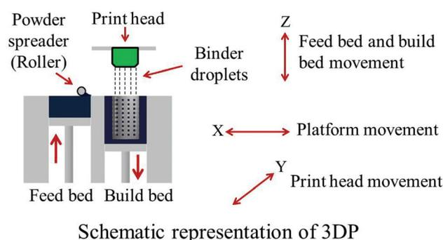
Fig. 1 Schematic representation of three dimensional printing (3DP).
