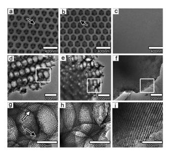
**Fig. 5** Typical SEM and TEM micrographs of macro-mesoporous titania films (a, d, g) without and (b, e, h) with graphene and pure mesoporous titania film (c, f, i). Reprinted with permission from ref. 78. Copyright 2010 American Chemical Society.
