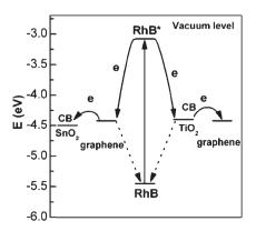
Fig. 7 The energy diagrams of RhB, graphene,  ${\rm TiO_2}$  and  ${\rm SnO_2}$ . Reprinted from ref. 59.
