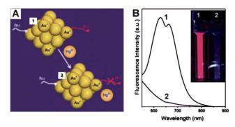
Fig. 4 (A) Schematic of Hg2+ sensing based on the fluorescence quenching of AuNCs resulting from high-affinity metallophilic Hg2+-Au+ bonds. (b) Photoemission spectra ( $\lambda_{ex} = 470 \text{ nm}$ ) and (inset) photographs under UV light (354 nm) of AuNCs (20 µM) in the (1) absence and (2) presence of Hg<sup>2+</sup> ions (50 µM). Reproduced with permission from ref. 65. Copyright 2009, RSC.
