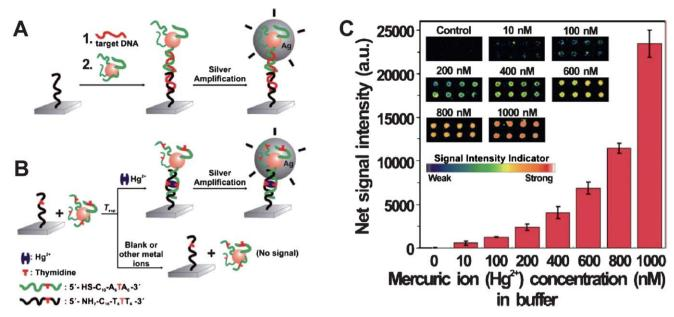
Fig. 3 (A) Conventional chip-based scanometric detection of target DNA using DNA-AuNPs; and (B) chip-based scanometric detection of  $Hg^{2+}$  using DNA-AuNPs. (C) Average scanometric signal intensity as a function of the  $Hg^{2+}$  concentration in buffer. The corresponding scanometric signal images are shown as an inset. The spot diameter is ~200  $\mu$ m. Reproduced with permission from ref. 49. Copyright 2008, ACS.
