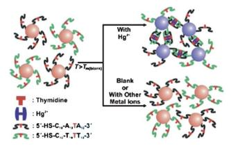
Fig. 2 Colorimetric detection of Hg<sup>2+</sup> based on DNA-modified AuNPs. Reproduced with permission from ref. 47. Copyright Wiley-VCH Verlag GmbH & Co.
