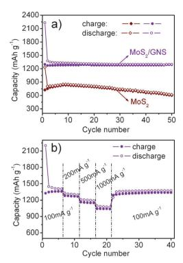
**Fig. 3** (a) Cycling behaviors of  $MoS_2$  and  $MoS_2/GNS$  at a current density of 100 mA  $g^{-1}$ . (b) Cycling behavior of  $MoS_2/GNS$  at various current densities.
