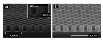
**Fig. 6** SEM images of (A) the hard silicon master with depth and width noted inset, and (B) the soft stamp cast obtained from photocuring the PMMS/TAC/BPDMA mixture. Reproduced by permission of WILEY-VCH from ref. 80: Campos *et al.*, *J. Adv. Mater.*, 2008, **20**, 3728–3733. DOI: 10.1002/adma.200800330.
