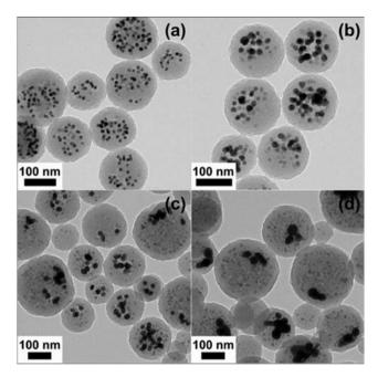
**Fig. 14** TEM images of Fe–Au hybrid organic–inorganic nanoparticles prepared by coencapsulation of MnFe<sub>2</sub>O<sub>4</sub> (10 wt% loading) with an average diameter of 13.0 nm and Au nanoparticles (19 wt% loading) of average diameter 13.0 nm (a), 18.0 nm (b), 24.0 nm (c), and 46.0 nm (d). Reproduced by permission of The American Chemical Society from ref. 89: van Berkel *et al.*, *Macromolecules*, 2009, **42**, 1425–1427. DOI: 10.1021/ma802849f. Copyright 2009 American Chemical Society.
