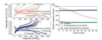
Fig. 3 (a) Galvanostatic charge—discharge curves of as-synthesized and carbon-decorated Fe<sub>3</sub>O<sub>4</sub> nanowires in lithium cells (charged at various C-rates from 0.1C to 5C but discharged at a constant rate of 0.1C) and (b) cycling performances of the Fe<sub>3</sub>O<sub>4</sub> nanowires before and after carbon decoration at 0.1C rate. For a comparison, data for a natural graphite electrode is also shown.
