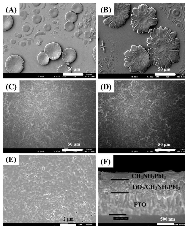
**Fig.2** Top-view SEM images of mesoporous TiO<sub>2</sub> films coated with inkjet printing perovskite from the precursor solution with a molar ratio of 1-x:1:x for PbI<sub>2</sub>, MAI, and MACl, respectively, at x=0 (a), x=0.3 (b), x=0.6 (c), x=0.9 (d), (e) x=0.6, the scale bar is 1  $\mu$ m; and the cross-sectional SEM image at x=0.6 (f).
