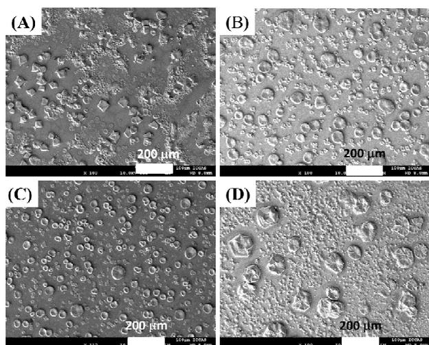
**Fig.1** Top-view SEM images of inkjet printed perovskite (on mesoscopic TiO<sub>2</sub> films) deposited at 25 °C (a), 40 °C (b), 50 °C (c), and 60 °C (d).
