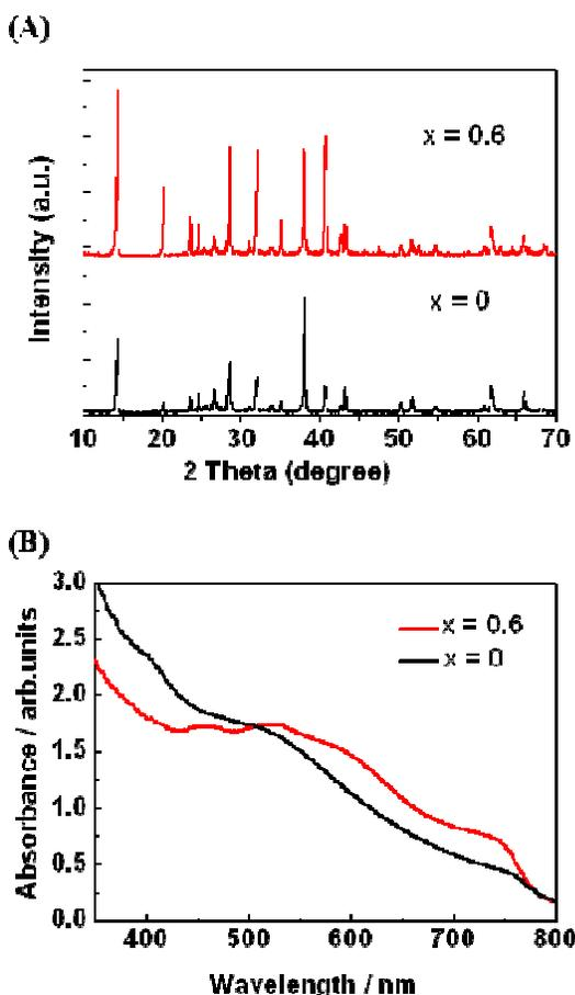
Fig.3 XRD diffraction patterns (a) and UV-vis spectra (b) of the perovskite-coated TiO<sub>2</sub> films prepared at x=0 and 0.6 from the precursor solution (the molar ratio of PbI<sub>2</sub>, MAI, and MACI is 1-x:1:x)
