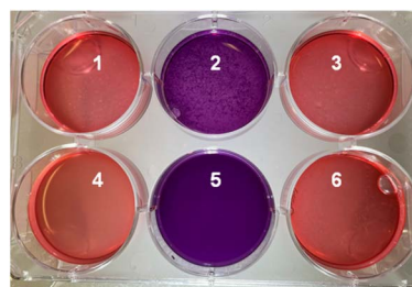
Fig. 12 Tests with pineapple juices and blackberry extracts. Sample 1 contains blackberry extract mixed with dilute HCl. Sample 2 contains blackberry extract mixed with SnCl 2 . Sample 3 contains blackberry extract. Sample 4 contains blackberry extract mixed with pineapple juice from a carton. (e) Sample 5 contains blackberry extract mixed with pineapple juice from a tin can (f) Sample 6 contains blackberry extract mixed with fresh pineapple juice.
